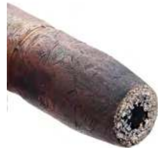
Nozzle fully clogged (not using E-WELD Nozzle)
