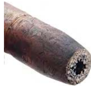
Nozzle fully clogged (not using E-WELD Nozzle)
