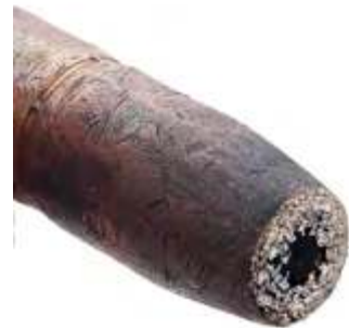
Nozzle fully clogged (not using E-WELD Nozzle)
