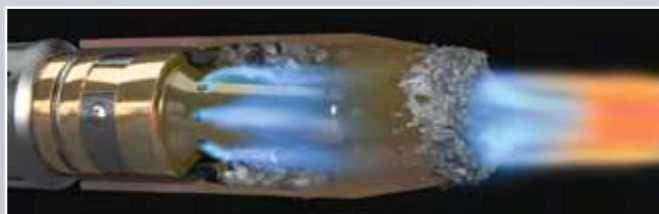
Spatter build up obstructs gas flow, resulting in inconsistent weld quality.
