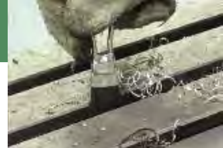
Removing chips from the slots of a milling machine.
