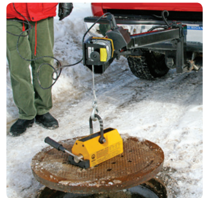
Pictured Right: Optional Front Bumper Adaptor (MCLBA12) for C-Channel bumpers
