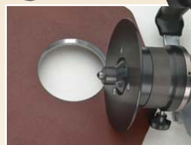
Above: LKF450 Multipurpose Beveling Machine. Bevel 30° or 45° and R2.5 radius
