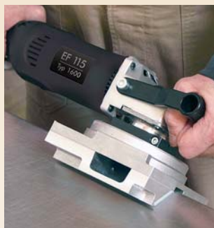
Above: EF 115 Deburring and Faceting Machine. Ideal for awkward, heavy parts, frame constructions or large sheets of metal.
