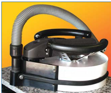
DS 301 with optional cowl for dry operation
