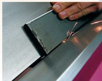
Above: EF 115 Deburring and Faceting Machine. Ideal for awkward, heavy parts, frame constructions or large sheets of metal.
