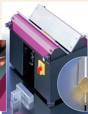
Above: LKF450 Multipurpose Beveling Machine. Bevel 30° or 45° and R2.5 radius
